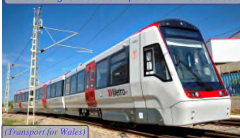
A Class 398 tram-train for Transport for Wales. Note the higher doors compared with the class 399
